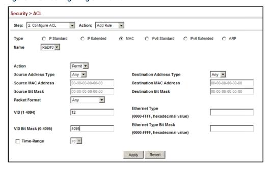
**CONFIGURING** Use the Security > ACL (Configure ACL - Add Rule - ARP) page to configure AN ARP ACL ACLs based on ARP message addresses. ARP Inspection can then use these ACLs to filter suspicious traffic (see "Configuring Global Settings for ARP Inspection" on page 372).
