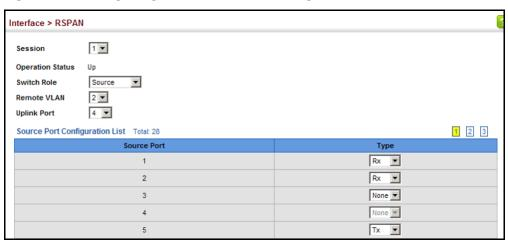
Figure 37: Configuring Remote Port Mirroring (Intermediate)
