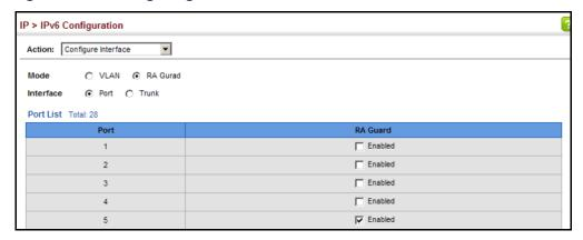
**CONFIGURING AN** Use the IP > IPv6 Configuration (Add IPv6 Address) page to configure an **IPv6 Address** IPv6 interface for management access over the network.
