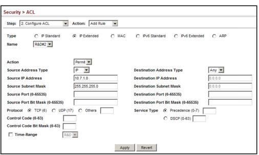
Figure 193: Configuring an Extended IPv4 ACL
