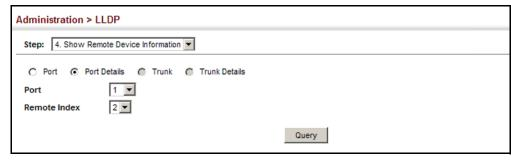
Figure 240: Displaying Remote Device Information for LLDP (Port Details)
