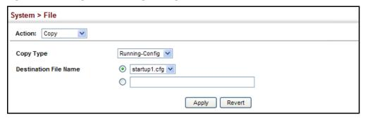
If you replaced a file currently used for startup and want to start using the new file, reboot the system via the System > Reset menu.
