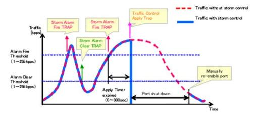
Figure 123: Storm Control by Shutting Down a Port
