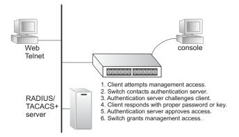
RADIUS uses UDP while TACACS+ uses TCP. UDP only offers best effort delivery, while TCP offers a more reliable connection-oriented transport. Also, note that RADIUS encrypts only the password in the access-request packet from the client to the server, while TACACS+ encrypts the entire body of the packet.
