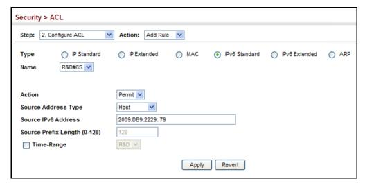
**CONFIGURING AN** Use the Security > ACL (Configure ACL - Add Rule - IPv6 Extended) page **EXTENDED IPv6 ACL** to configure an Extended IPv6 ACL.
