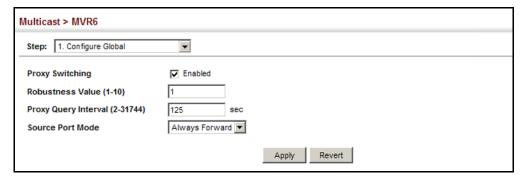
**CONFIGURING MVR6** Use the Multicast > MVR6 (Configure Domain) page to enable MVR6 **DOMAIN SETTINGS** globally on the switch, and select the VLAN that will serve as the sole channel for common multicast streams supported by the service provider.
