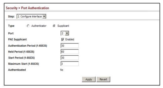
**DISPLAYING** Use the Security > Port Authentication (Show Statistics) page to display **802.1X STATISTICS** statistics for dot1x protocol exchanges for any port.
