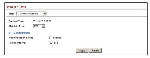
**CONFIGURING** Use the System > Time (Configure Time Server) pages to specify the IP TIME SERVERS address for NTP/SNTP time servers, or to set the authentication key for NTP time servers.
