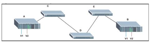
Without VLAN trunking, you would have to configure VLANs 1 and 2 on all intermediate switches – C, D and E; otherwise these switches would drop any frames with unknown VLAN group tags. However, by enabling VLAN trunking on the intermediate switch ports along the path
