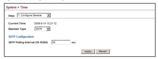
**CONFIGURING NTP** Use the System > Time (Configure General - NTP) page to configure NTP authentication and show the polling interval at which the switch will query the specified time servers.
