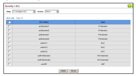
**CONFIGURING A** Use the Security > ACL (Configure ACL - Add Rule - IP Standard) page to **STANDARD IPv4 ACL** configure a Standard IPv4 ACL.
