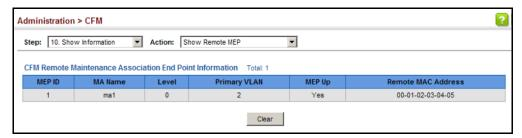
**DISPLAYING DETAILS** Use the Administration > CFM > Show Information (Show Remote MEP FOR REMOTE MEPs Details) page to show detailed information for MEPs located on other devices which have been discovered through continuity check messages, or statically configured in the MEP database and verified through cross-check messages.
