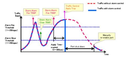
Figure 411: Storm Control by Shutting Down a Port
