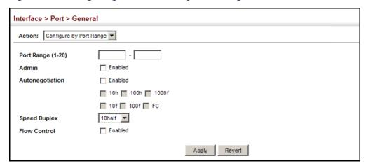
**DISPLAYING** Use the Interface > Port > General (Show Information) page to display the CONNECTION STATUS current connection status, including link state, speed/duplex mode, flow control, and auto-negotiation.
