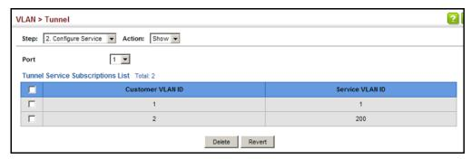
The preceding example sets the SVID to 99 in the outer tag for egress packets exiting port 1 when the packet's CVID is 2. For a more detailed example, see the switchport dot1q-tunnel service match cvid command on page 1135.
