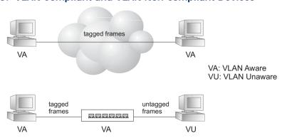
**VLAN Classification** – When the switch receives a frame, it classifies the frame in one of two ways. If the frame is untagged, the switch assigns the frame to an associated VLAN (based on the default VLAN ID of the receiving port). But if the frame is tagged, the switch uses the tagged VLAN ID to identify the port broadcast domain of the frame.
