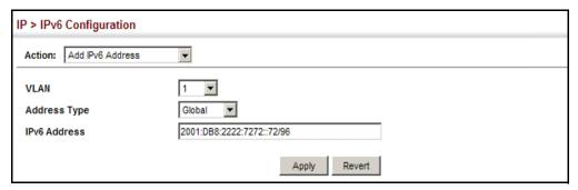
**SHOWING** Use the IP > IPv6 Configuration (Show IPv6 Address) page to display the **IPv6 Addresses** IPv6 addresses assigned to an interface.
