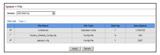
To start using the new firmware or configuration settings, reboot the system via the System > Reset menu.
